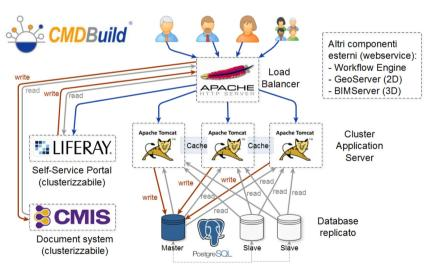
efficient thanks to the possibility of using the "slave" instances of PostgreSQL for only-read operations, distributing in this way the work load among the available databases.
