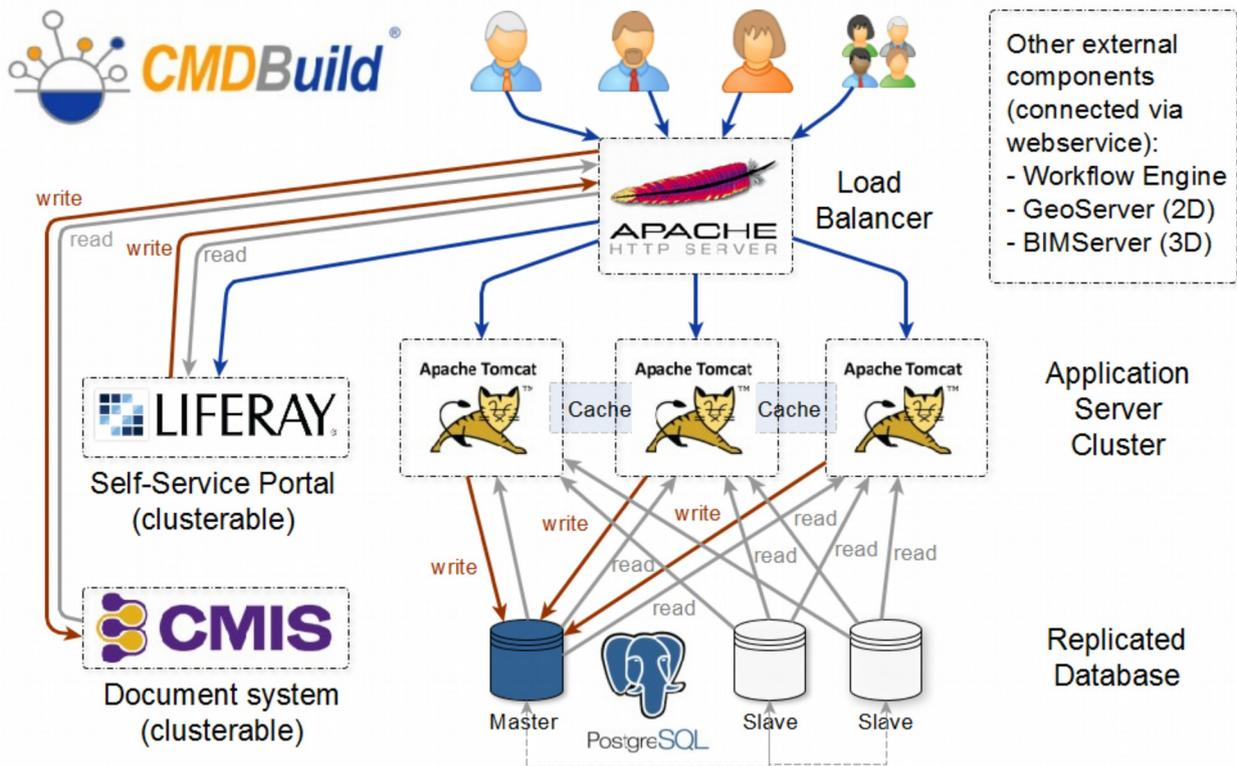
In the example above the load balancer has been made by the Apache webserver.
